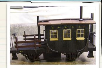
"I needed a battery car directly behind the tender. The side-dump ore cars this locomotive pulls were too small. I had an unused Aristocraft caboose, but it looked wrong at the head of the train. I cut one third of the body out, including the cupola to lower the profile, and turned it into a "transfer" caboose."
